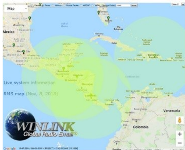
Figure 1 RMS nodes installed in beneficiary countries and possible coverage and Winlink network scheme
